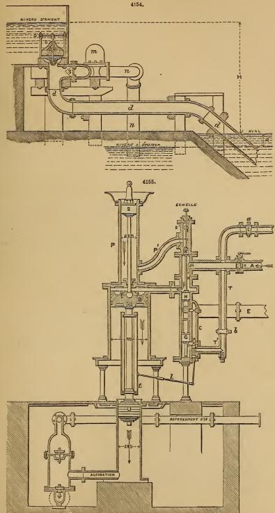
With respect to the mode of action of the water, these engines are divided into two classes : single-action and double-action engines ; the former are vertical, the latter horizontal. Direct and
